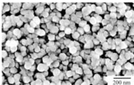
Figure 2. An SEM image of the CdS film deposited from run 1 in Table 1.
